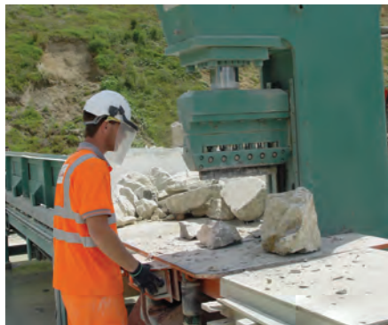
From top to bottom: ● The Aldi store in Maidstone makes a feature of Kentish Ragstone walling from the local quarry. ● The 3.2m Van Voorden primary saw. ● The cut taking the quarry into the new area to be worked. ● The Steinex cropper used to produce walling stone. ● Bags of walling stone waiting for delivery.
